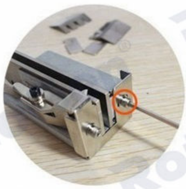
4. Loosen the screw on the right side of the front bezel. (not screw out)
